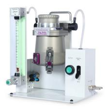
A precise and calibrated flow meter ranging from 0.1 to 4.0LPM with a large scale for precision and ease of reading is mounted on the Anesthesia module.
